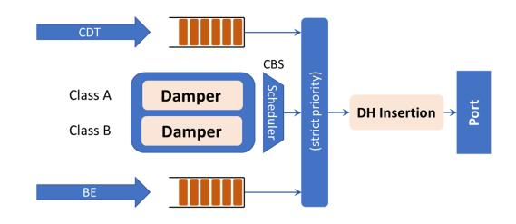
Damper Header inserted on the transmission line.
