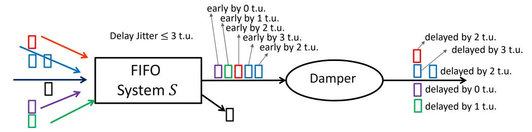
Damper delays a packet by "earliness" read from packet header.
