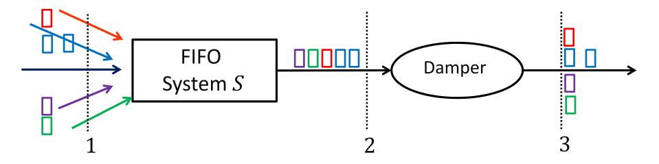
Delay jitter  $1 \rightarrow 3$  is 0 in theory; in practice, a small residual delay jitter  $\leq \Delta$  (in true time):
