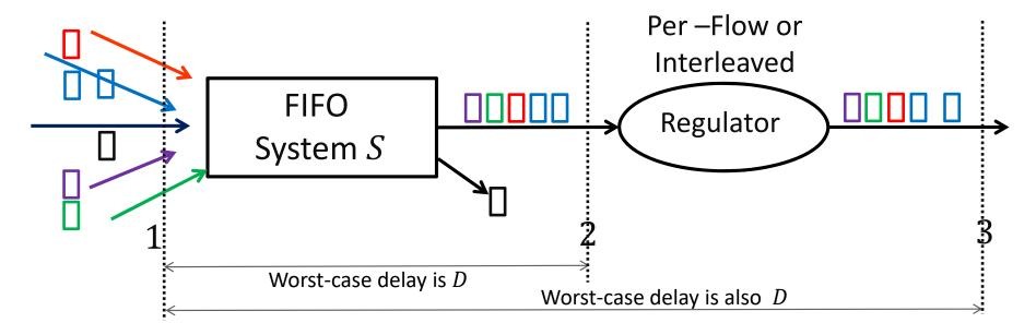
Assume S is FIFO per flow (per-flow regulator) or globally (interleaved regulator).
